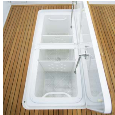
■ Fish and stowage wells are insulated, heavily gasketed and fitted with locking hatches that are supported with stainless-steel gas struts.
